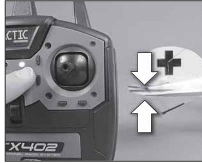
Before flight, center elevator control surface with elevator trim adjustment.
