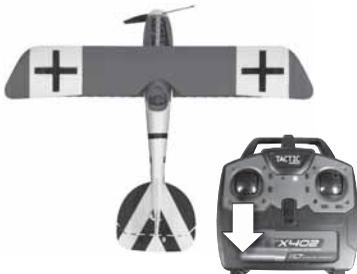
Throttle control stick is in the low or minimum position.
