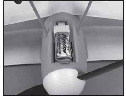
Press battery into place to secure.
