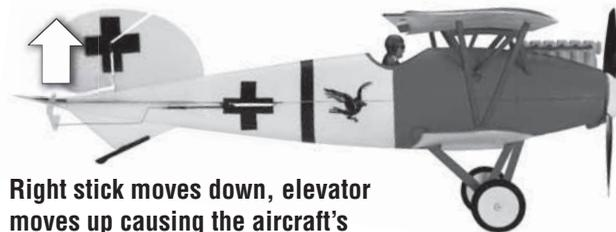
Right stick moves down, elevator moves up causing the aircraft's nose to pitch up, gaining altitude.
