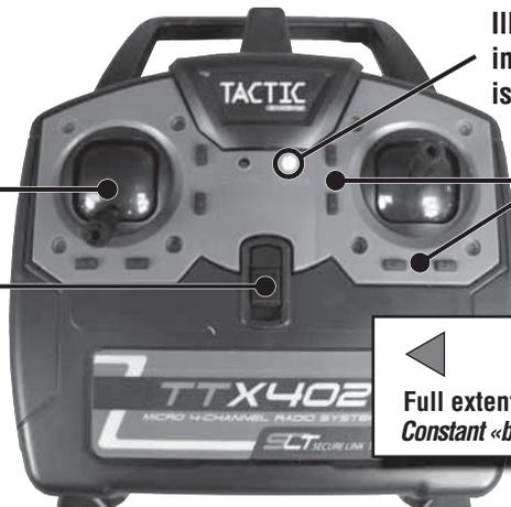
Illuminated red light indicates the TTX402 is powered and transmitting.
