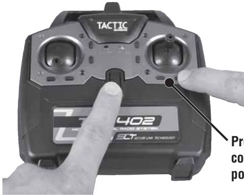
Press and hold one of the corresponding control surface trim buttons and cycle the power to reverse any control surface.
