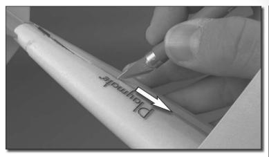
1. Use the tip of a hobby knife (a paring knife would suffice) to cut the side seam of the Playmate (either side may be cut). Be careful to only insert the tip of the knife into the seam as penetrating too far may damage the internal components of the Playmate.
