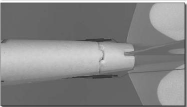
7. Add a small amount of foam-safe CA to the previously cut seam and close the Playmate Fuselage Halves, being sure not to bind the tail control linkages.
