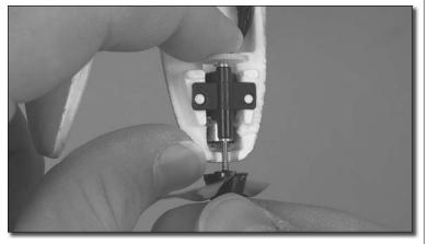
6. Using your index finger (or pliers) to hold the spur gear and shaft into the forward position, press the propeller onto the shaft and hold for one minute. Inspect the fit and make sure the propeller is secure and that the spur gear is meshed with the pinion.
