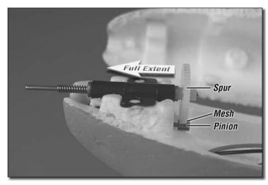
4. Slide the spur gear onto the pinion gear and move the shaft forward to the full extent. Next, re-install the spring onto the prop shaft.
