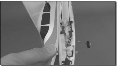
2. Open the fuselage of the Playmate by using the un-cut seam as a hinge.
