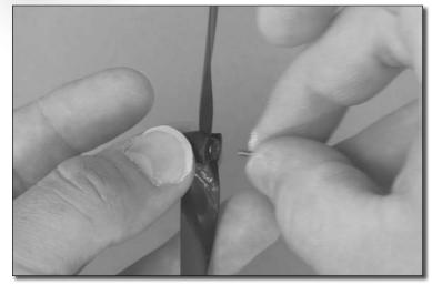
3. If the spring is still attached to the propeller, carefully remove it from the propeller. Do not to stretch the spring. If you no longer have the spring, contact Product Support at (217) 398-8970, extension 5.
