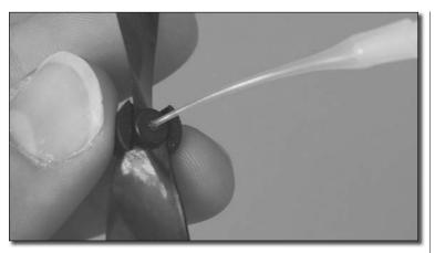
5. Apply a small amount of CA into the small mounting hole in the propeller. Quickly move onto step 6 before the CA fully cures.
