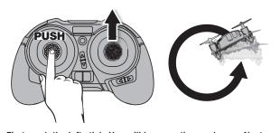
First, push the left stick. You will hear continuous beeps. Next, move the right stick any direction and the Proto-X will flip that direction.
