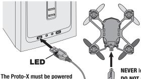
Plug the charger into a USB port and the Proto-X as shown. (The battery connector will only fit in one way. Do not force the connectors together.)
