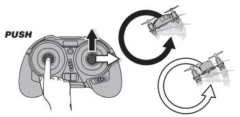
First, push the left stick. You will hear continuous beeps. Next, move the right stick any direction and the Proto-X will flip that direction.
