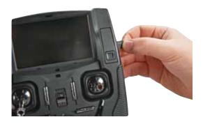
You can also install the micro memory card in your transmitter, reformat it, and capture video using the transmitter. Your transmitter will then be able to read and play the file - but **NOT** your computer.
