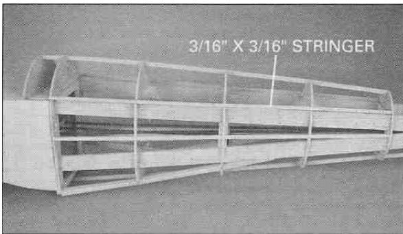
□ 2. Add a stringer to the fuselage from former DT to HT. Use the supplied 3/16" x 3/16" x 24" balsa sticks. Cut notches in top formers DT, ET, FT, GT and HT, and add a stringer to each side as shown in the photo above. This will provide a gluing surface where the top sheeting meets the side sheeting.
