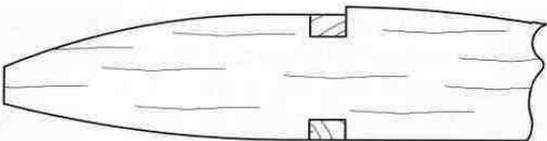
6. Test fit the top 1/8" x 3/16" spar into place. If it doesn't fit properly, enlarge the notches in the ribs so the spar fits completely in the notch. This is important so the .040" LE sheet will blend with the rear portion of the rib. Glue the spar in place with thin CA.
