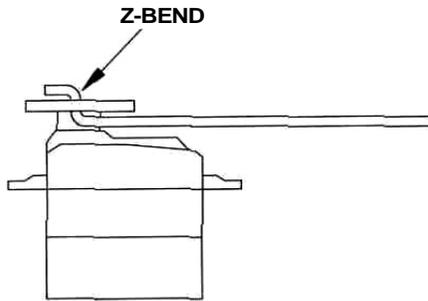
3. When you have the forward part of the pushrod bent and attached/ slide the wire into the tube from the front. Then mount the servos using double-sided tape.
