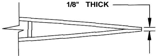
4. Taper the 1/4" sq. longerons at the rear of the fuselage with a sanding block so when the bulkheads are installed the tail will pull together to measure about 1/8" thick.
