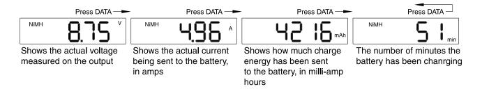
Note that when the LCD shows the battery's voltage during charge, the reading will seem slightly higher than normal. This is due to the loading effect of the charger, and is normal. A higher load will skew the reading more than a smaller load. When fast charge is finished, battery voltage readings will be more accurate.
