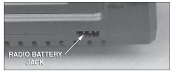
RADIO BATTERY JACK: A unique jack is located on the front edge of the charger, for charging of NiCd or NiMH 4 or 5 cell receiver batteries for nitro vehicles, or even 8 cell transmitter batteries! This jack is universal – compatible with Futaba-J, Airtronics-Z, Hitec, JR, and Spektrum receiver battery connectors, and BEC type connectors.
