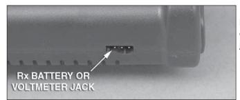
Rx BATTERY OR VOLTMETER JACK: A unique jack is located on the front edge of the charger, for charging of NiCd or NiMH 4 or 5 cell receiver batteries for nitro vehicles. This jack is universal – compatible with Futaba-J, Airtronics-Z, Hitec, JR, and Spektrum receiver battery connectors, and BEC type connectors.
