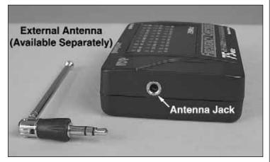
The 75MHz Frequency Checker has a built-in antenna which is designed to receive transmitter signals from within a 300 foot radius. If a greater range is desired, an external antenna is available separately (DTXP3111). Contact your local hobby shop for details. Using the external antenna can extend the Frequency Checker's range to a radius of 1000 feet. It's best to point the antenna skyward for best reception.
