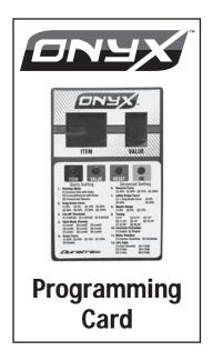
The Onyx Programming Card is a handheld device that allows users to easily adjust the features of the Onyx 80A and 120A brushless ESCs. The programmer is small and lightweight, making it highly portable and easy to take anywhere. This programmer allows the user to fine-tune the adjustable features of the ESC and is also great for quick, easy setup changes while at the track.
