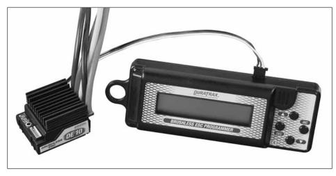
Connect the ESC to the programmer by plugging the ESC lead into jack located on the top of the programmer.
