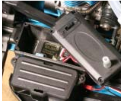
Tucked inside of the radio box is DuraTrax's three-channel RX-300F FM receiver. Next to the Rx box is the four-cell battery holder box.
