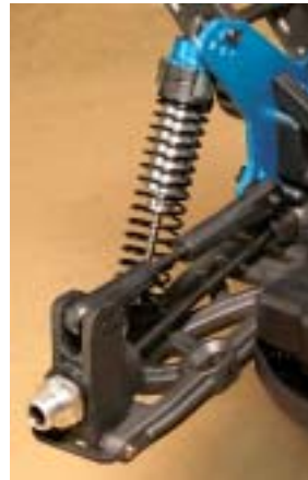
The rear hub offers several mounting locations for the rear adjustable tie-rod to alter the buggy's roll. Notice how the arm features a molded support that wraps around the hub to connect the two sides of the pivot to reduce flex.
