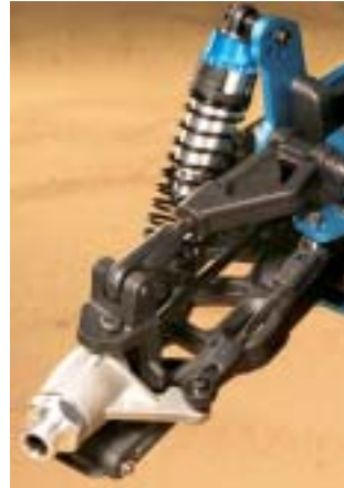
Here is a good look at the cast aluminum knuckles that support the steel axle and 17mm wheel hex. Bulky C-hubs mate up to the knuckle and pivot on E-clip-retained hinge pins. The upper arms are adjustable to alter camber.
