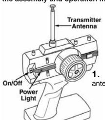
**1.** Install the transmitter antenna into the transmitter.
