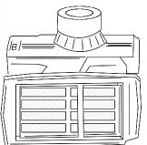
**2.** Install (8) "AA" batteries into the transmitter. Check to make sure the red power light glows when the transmitter is on.
