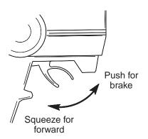
**5.** Make sure the throttle opens all the way when the throttle is applied on the transmitter. Make sure the brakes work adequately when the trigger is pushed forward.
