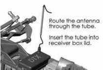
**3.** Install the receiver antenna tube. Secure the excess wire to the tube using tape. **DO NOT CUT THE ANTENNA WIRE.**
