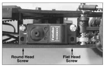
☐ 6. Install the steering servo onto the chassis from underneath using a 3x10mm flat head, self-tapping screw in the front hole which is countersunk; and a 3x10mm round head, self-tapping screw in the slotted rear mounting hole. Route the steering servo wire through the slotted hole between the steering servo and the receiver battery holder.
