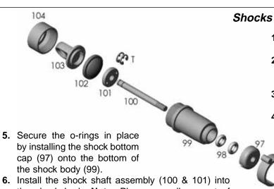
1. Install one 2mm e-clip (T) onto the lower groove in the shock shaft (100).
