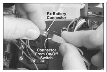
☐ 5. Plug the male end of the wire from the receiver (RX) battery into the female end from the on/off switch.
