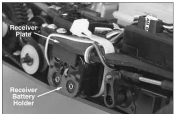
☐ 4. It may be necessary to loosen the radio plate to remove the receiver battery holder. Install 4 "AA" batteries (included) into the receiver battery holder in the configuration molded into the battery holder. Install the receiver battery back into the receiver battery holder as shown. Make sure to re-tighten the radio plate screws once the receiver battery is in place.
