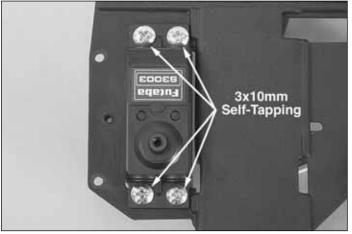
☐ 3. Install the throttle/brake servo into the slot next to the fuel tank. Place the two servo mount blocks onto the bottom of the radio plate. Then install the four 3x10mm self-tapping screws through the servo into the servo mounts. Route the servo wire through the slotted hole between the servo and the receiver battery holder.
