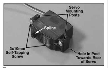
☐ 5. Using two 3x10mm self-tapping screws, install the two servo mounting posts onto the steering servo as shown (note location of servo spline). Note that the hole in the bottom of the servo mounting posts are off-center. Install the posts with the hole in the bottom of the post as shown in the photo. This is to help prevent the servo from hitting the center belt.
