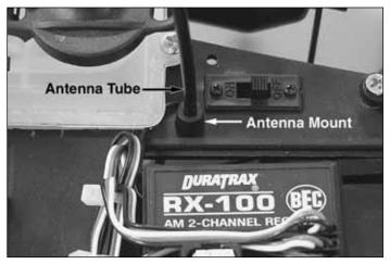
☐ 2. Remove the twist-tie from around the receiver antenna wire. Run the length of the antenna wire through your fingers to help straighten the wire out. This will make it easier to get the wire through the antenna tube. Slide the antenna wire through the antenna tube. Press the antenna tube into the antenna mount molded into the top of the radio plate.
