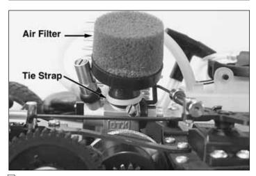
1. Install the air filter onto the carburetor. Using the included tie-strap, secure the air filter to the carburetor. Cut off any excess portion of the tie-strap to avoid interference.
