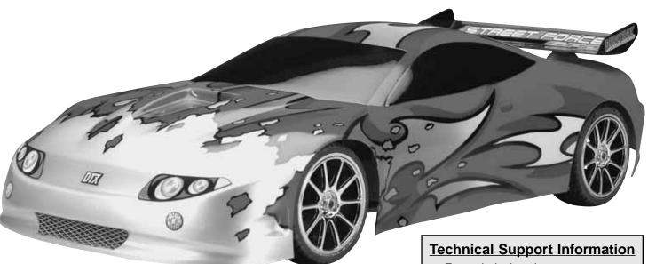
Length: 16.5" [435mm] Width: 7.7" [195mm] Height: 4.6" [115mm] Weight: 3.1 lb [1.4kg] Wheelbase: 10.1" [255mm] For technical assistance, contact:
