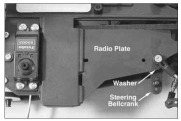
4. Reinstall the radio plate onto the chassis. Make sure to reinstall the washer between the steering bellcrank and the radio plate.
