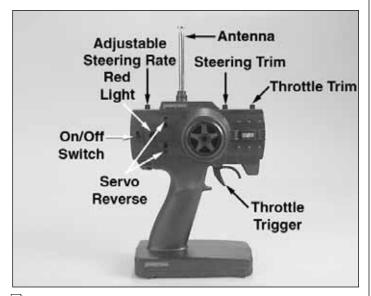
☐ 6. Install the transmitter antenna by screwing it into the hole on the top of the transmitter. Give the antenna a mild tug to make sure that it is properly secured in the transmitter.
