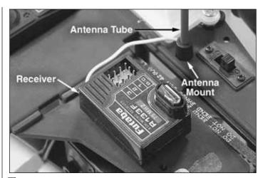
☐ 7. Install the receiver using the included double-sided tape onto the top of the radio plate as shown. Run the length of the antenna wire through your fingers to help straighten the wire out. This will make it easier to get the wire through the antenna tube. Slide the antenna wire through the antenna tube. Press the antenna tube into the antenna mount molded into the top of the radio plate.
