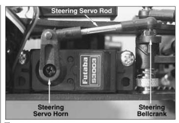
☐ 13. Snap one end of the rod onto the steering servo horn. Snap the other end onto the steering arm. Turn the transmitter on and center the steering trims. Install the steering servo horn onto the steering servo as shown. Then turn the transmitter and receiver off.
