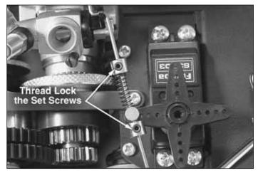
☐ 16. Make sure the carburetor is at the idle setting (refer to the throttle stop screw, page 10). Then, install the second rod collar onto the end of the throttle linkage rod. The rod collar should slide up against the throttle linkage rod connector as shown.
