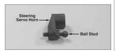
☐ 11. Thread the ball stud into the correct steering servo horn (included) for your steering servo as shown. Test fit the servo horn onto your servo first to make sure it is the correct one.
