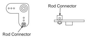
☐ 14. Install the rod connector into the hole farthest away from the center on the short servo horn (included). **Note:**This hole is slightly enlarged. Place the small metal washer and 2mm nut onto the bottom of the rod connector. Make sure not to over-tighten the nut. The rod connector must swivel freely. Apply a small amount of thread lock onto the nut to prevent it from falling off during running.
