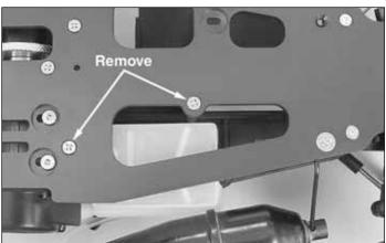
1. Remove the radio plate from the chassis by removing the 9 screws as indicated in the above photos.
