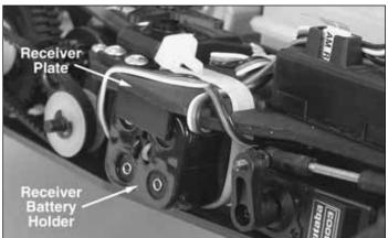
☐ 10. Install the four "AA" batteries into the receiver battery holder as shown. It may be necessary to loosen the radio plate slightly to fit the receiver battery in. Make sure to re-tighten the radio plate screws once the receiver battery is installed.
