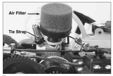
20. Install the air filter onto the carburetor. Using the included tie-strap, secure the air filter to the carburetor. Cut off any excess portion of the tie-strap to avoid interference.
