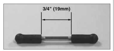
12. Thread the two ball ends onto the steel rod. There should be 19mm or 3/4" between the two ball ends.
