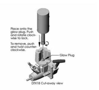
□ 6. Install the glow starter onto the glow plug and gently press the top of the glow starter down and turn in a clockwise direction. This will lock the glow starter onto the glow plug. To remove the glow starter, gently press down on the top of the glow starter and turn counter clockwise.
