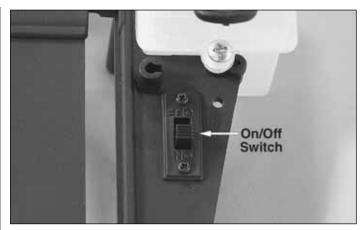
□ 2. Install the on/off switch into the slot in front of the fuel tank. Remove the face plate from the switch, then install the switch up through the bottom of the radio plate, and then install the face plate onto the top of the radio plate. Re-install the two screws through the face plate and into the switch to secure it to the radio plate. Be careful to put the switch plate on correctly with respect to on and off switch positions.
