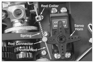
☐ 15. Locate the small rod with a z-bend at one end. Install the z-bend end of the rod into the lower hole of the throttle arm on the carburetor. Turn the transmitter on again and
