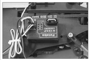
☐ 9. Plug the switch wire into the battery ("BATT") slot on the receiver. Plug the steering servo and throttle servo wires into the receiver. See your radio instructions to determine which channel is steering and which is throttle.
