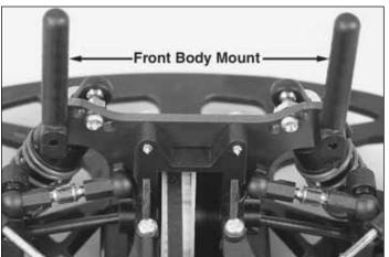
9. Raise the body posts to the upright position. Notice there is a molded pin that fits into a hole in the shock tower. This is to keep the body posts from swiveling during running. Tighten the screws in the body posts, making sure that the posts pull tight against the shock towers. You will have to remove the screws in the tops of the front shocks to get to the front body mount screws.
