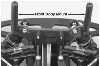
☐ 21. Raise the body posts to the upright position. Notice there is a molded pin that fits into a hole in the shock tower. This is to keep the body posts from swiveling during running. Tighten the screws in the body posts, making sure that the posts pull tight against the shock towers. You will have to remove the screws in the tops of the front shocks to get to the front body mount screws.
