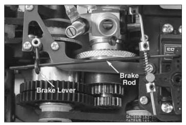
☐ 18. Lift the throttle linkage servo horn off of the servo. Install the remaining z-bend wire from the bottom into the hole farthest from the center of the servo horn. **Note:** This hole is slightly enlarged. Slide the threaded end of the brake linkage rod through the brake lever.
