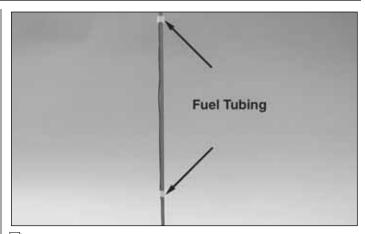
☐ 3. Frequently, there will be leftover wire protruding from the antenna tube. **Do not cut or coil the antenna!** Cut two pieces of fuel tubing 1/8" long and slide them over the outside of the antenna tube and wire. This is to help hold the excess antenna onto the tube and avoid getting the antenna wire cut in a roll over. Note the placement of the fuel tubing on the antenna tube.
