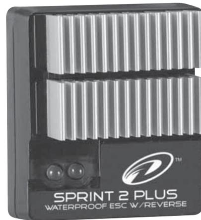
**NOTE:** The Sprint 2 has built-in circuitry to sense an excessive heating condition caused by current overload. If the ESC overheats, it will automatically shut down, as indicated by flashing red and green LEDs. This is to protect all on-board components and prevent permanent damage from occurring. The ESC can again be used once the internal temperature returns to an acceptable level. Reset by cycling the power.
