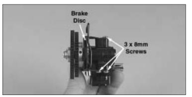
20) Reattach the brake assembly to the gearbox using the three 3 x 8mm screws making certain that the brake disc is between the brake plates.
