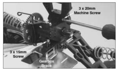
12) Remove the rear shock tower by removing the 3 x 20mm machine screw. Remove the 3 x 15mm screw from the gearbox brace.
