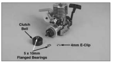
3) Remove the 4mm E-clip from the end of the pilot shaft and remove the clutch bell and two flanged 5x10mm clutch bell bearings.
