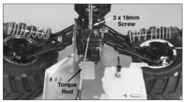
10) Detach the torque rod from the brake assembly by removing the 3 x 18mm screw.
