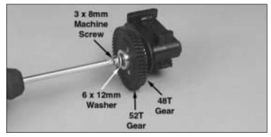
19) Place the 48 tooth spur gear onto the main gear shaft so that the attached aluminum clutch drum covers the clutch assembly. Follow that with the 52 tooth spur gear (screwheads facing away from the gearbox) and a 6 x 12mm washer onto the main gear shaft. Apply a small amount of thread lock to the 4 x 8mm machine screw and install it into the end of the main gear shaft as shown in the photo.
