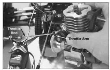
27) Reattach the throttle rod to the carburetor. This is done by inserting the z-bend of the throttle rod through the outer hole of the throttle arm. Rotate the engine into place.
