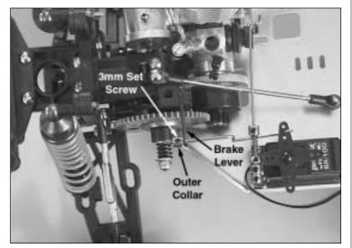
1) Disconnect the brake rod by loosening the 3mm set screw and sliding the outer collar off of the brake rod.
