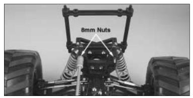
8) Detach the rear shock tops by removing the 3mm nuts. Lean the shocks to either side.
