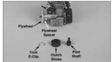
4) Remove the 7mm E-clip and gently remove the clutch shoes with clutch spring attached (note direction). Remove the pilot shaft with a 10mm wrench or socket. Use a crankshaft locking tool (not included) to "lock" the crankshaft in place and prevent it from rotating while removing the pilot shaft. A crankshaft locking tool is available from
