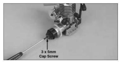
7) Remove the 5 x 10mm flanged bearing from the old clutch bell and install it into the end of the new clutch bell and slide it onto the pilot shaft. Apply a small amount of thread lock to the 3 x 6mm cap screw and insert into the end of the pilot shaft to secure the clutch bell to the engine.
