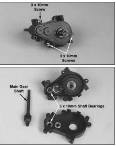
16) Remove the three 3 x 10mm screws holding the gearbox halves together. Carefully open the gearbox (make sure the gears do not fall out while separating the halves). Remove the main gear shaft and both 5 x 10mm shaft bearings.
