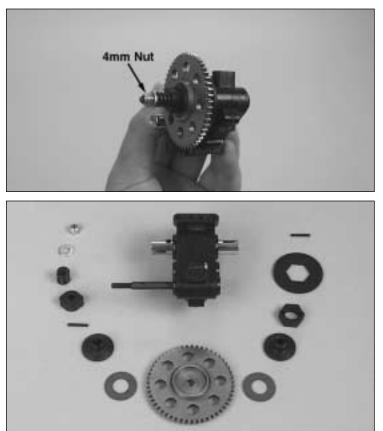
15) Remove the 4mm nut from the main gear shaft. Remove the slipper clutch components and spur gear from the main gear shaft.
