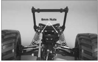
26) Reattach the shocks to the shock tower by re-installing the 3mm nuts.
