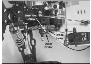
29) Slide the brake rod through the brake lever and replace the metal collar. DO NOT tighten the collar until we are sure that the brake is set up properly. Follow this sequence:
