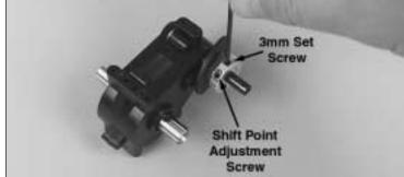
18) Slide the brake disc onto the 2-speed clutch. Slide the 2-speed clutch and brake disc onto the main gear shaft. Secure the 2-speed clutch to the main gear shaft with the 3mm set screw. Ensure that the 3mm screw seats on the flat spot on the main gear shaft. NOTE: There is a 4mm set screw for adjusting the shift point on the 2-speed. This screws into the clutch at an angle. Do not mistake this for the screw that secures the clutch to the main gear shaft.
