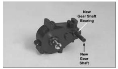
17) Install the new 6 x 10mm main gear shaft bearings into the gearbox halves. Install the new main gear shaft. Reassemble the gearbox using the three  $3 \times 10$ mm screws.
