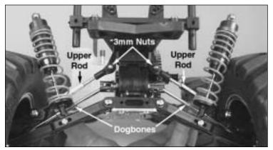
9) Detach the rear upper rods by removing the 3mm nuts. This will enable you to remove the rear dogbones.
