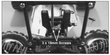
11) Remove the body mount assembly by removing the two 3 x 18mm screws.
