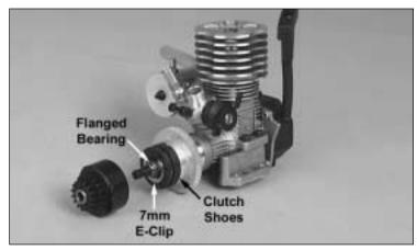
6) Reinstall the clutch shoes with spring attached (note direction of shoes with the narrow side towards the front of the the crankshaft), the 7mm E-clip, and the 5 x 10mm flanged bearing.
