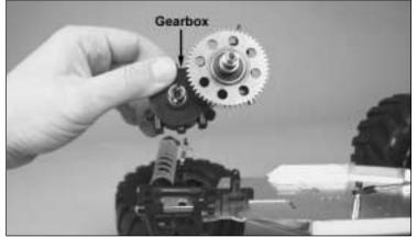
13) Remove the gearbox by removing the four 3 x 10mm screws.
