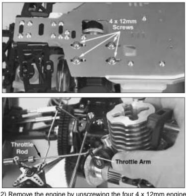
2) Remove the engine by unscrewing the four  $4 \times 12$ mm engine mounting screws. Disconnect the throttle rod from the carburetor by rotating the engine.
