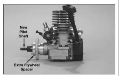
5) Add the extra flywheel spacer to the crankshaft. The pins on the flywheel should insert into the holes of the flywheel spacer. Install the new pilot shaft. The pilot shaft must be tight to prevent it from loosening while running the vehicle. It is additionally suggested that you use thread lock (not included) on the crankshaft to help prevent the pilot shaft from loosening. **Note:** Remove the crankshaft locking tool when this step is completed.
