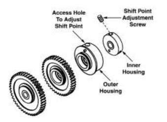
3) Rotate the outer housing back and forth until you can see a small set screw on the inner housing. This set screw does not go straight down into the inner housing, it is set at an angle. This is the adjustment screw for the shift point.
