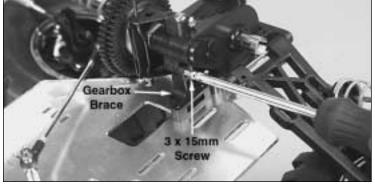
21) Reattach the gearbox to the chassis using the four 3 x 10mm screws and to the gearbox brace using the 3 x 15mm screw.
