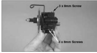
14) Remove the brake assembly from the gearbox by removing the three  $3 \times 8$ mm screws.
