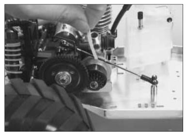
28) Reattach engine to the chassis using the four  $4 \times 12$ mm engine mounting screws, using threadlock on the screws. DO NOT tighten them completely. Make sure the gears mesh correctly by placing a single piece of paper between the 15T clutch bell gear and the 52T spur gear. Push the gears as close together as possible, then rotate the gears to remove the paper. If the paper tears, the gear mesh is too tight. Tighten the  $4 \times 12$ mm engine mounting screws.
