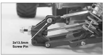
5) Remove the 3x13.5mm screw pin that holds the left, upper (camber) rod to the left, rear hub. Set aside the left swing shaft ("dogbone")
