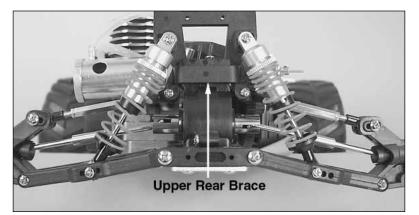
18) Slide the upper rear brace into place under the rear shock tower. Place the body mount assembly on top of the rear shock tower and reattach with two 3x15mm self-tapping screws. **Note:** Make sure that the screws go through the shock tower and the upper brace and into the transmission housing.
