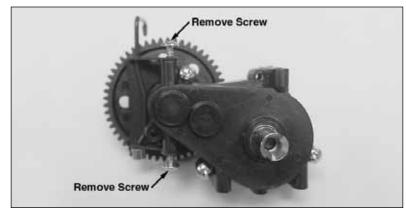
8) Now the transmission housing can be separated from the rest of the vehicle. Remove the two 3x8mm screws that hold the brake brace to the transmission housing. NOTE: Do not remove the third screw that holds the brake brace to the transmission housing.
