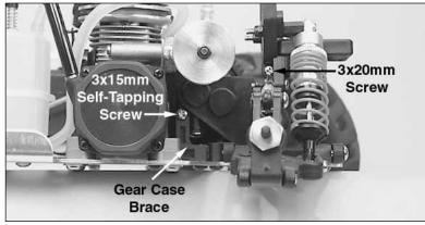
3) Remove the 3x20mm screw that holds the shock tower to the transmission housing and the 3x15mm self-tapping screw that holds the gear case brace to the transmission housing as shown in the photo.
