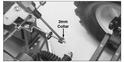
7) With a 1.5mm allen wrench, loosen the 3x3mm set screw in the 2mm collar from the brake rod and set the collar aside.
