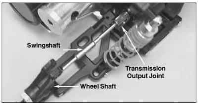
16) Insert the two swing shafts ("dogbones") between the transmission output joints and the rear wheel shafts (axles). Reattach the upper rod with the 3x13.5mm screw pin. **NOTE:** Make sure that you place the screw pin in from the rear of the vehicle and place it into the outer hole.
