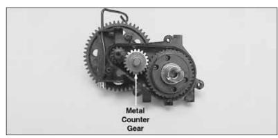
10) Lay the transmission flat on your workbench as shown in the photo and carefully slide the two transmission halves apart. Remove
