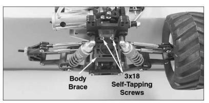
2) Remove the two 3x18mm self tapping screws holding the body brace to the transmission housing. Set aside the body mount/body brace assembly.
