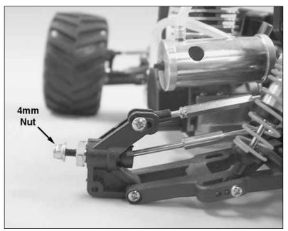
1) Remove the left rear wheel by removing the 4mm nut with the 7mm socket of the 4-way wrench that was supplied with your kit.
