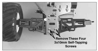
6) Remove the four 3x10mm self-tapping screws that hold the transmission housing to the chassis as shown in the photo.
