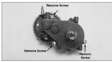
9) Remove the three 3x8mm self-tapping screws that hold the two halves of the transmission housing together.
