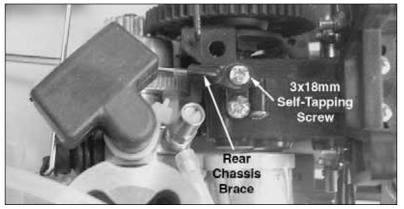
4) Remove the 3x18mm self-tapping screw that holds the rear chassis brace to the transmission housing.
