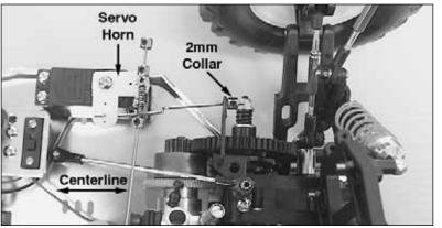
14) Align the throttle servo horn with the centerline of the chassis, as shown. Position the brake lever perpindicular to the centerline of the chassis. Place the 2mm collar onto the brake rod such that it is 2mm (1/16") away from the brake lever. With a 1.5mm allen wrench, tighten the 3x3mm set screw to hold the collar in place.
