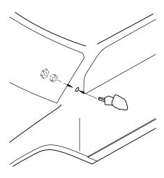
☐ 16. Drill one 1/8" (3mm) hole in each side of the body using the molded-in dimple as a guide. Install the mirrors as shown with the collars and nuts provided.
