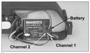
☐ 15. Plug the steering servo, throttle servo and switch into the receiver. See your radio instructions to determine which channel is steering and which is throttle. The switch plugs into the battery socket.
