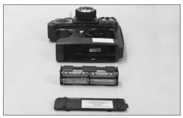
☐ 10. Slide open the battery door on the bottom of the transmitter and remove the transmitter battery holder. Place 8 "AA" batteries (included) into the holder in the configuration molded into the plastic on the battery holder. Re-install the transmitter battery holder into the transmitter and re-install the battery door.
