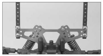
☐ 6. Remove the lower screw from each of the body posts so that the posts can be placed upright. Reinstall the screw through the shock tower into the body post as shown. The height of the body can be adjusted by raising or lowering the posts on the shock tower.
