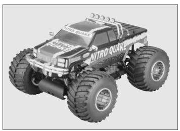
☐ 17. Remove the body clips from the parts bag. Place the body onto the body mounts. On each body mount place a body clip.
