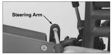
☐ 26. Loosen the screw in the bottom of the steering arm on the servo saver enough for the linkage rod to slide through the metal rod connector.
