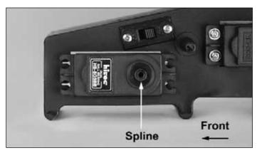
☐ 7. Place the high torque steering servo into the radio tray. Note the direction of the servo spline when installing. Run the servo lead through the hole in the side of the radio box.
