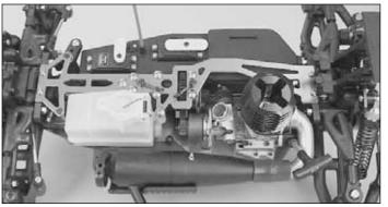
☐ 22. Re-install the radio box back onto the chassis. Use the (8) 3x15mm flathead self tapping screws that you removed earlier to secure the radio box back onto the chassis. Refer to the picture in step 2 on page 6.
