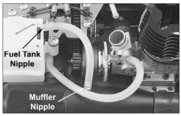
□ 39.Install one end of the 4" (100mm) piece of fuel tubing onto the nipple next to the fuel tank lid and the other end on the nipple on the muffler.
