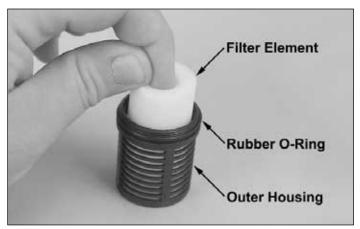
☐ 40. Assemble the air filter. Slide the large rubber Oring around the threads of the outer housing. The Oring will help seal the air filter housing together.
