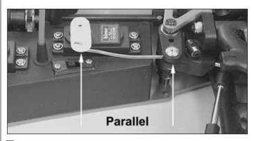
☐ 27. Remove the screw from the steering servo horn. Slide the steering linkage rod through the hole in the linkage rod connector in the steering arm. Place the servo horn back onto the servo. When placing the horn onto the servo, the horn and the steering arm should be parallel as shown in the photo. Note: Do not screw the servo horn down yet, the servos will need to be centered after assembly is completed.
