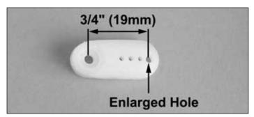
☐ 24. Remove the servo horn from steering servo. Enlarge the hole 3/4" (19mm) away from the center of the horn with a 5/64" (2mm) drill or a hobby knife.
