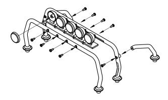
☐ 51. Assemble the rollbar as shown using ten 2.6 x 6mm self-tapping screws.
