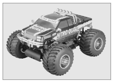
☐ 55. Remove the body clips from the parts bag. Place the body onto the body mounts. On each body mount place a body clip.
