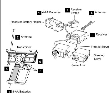
Before installing the radio system in the pre-built DuraTrax Nitro Quake read the manufacturer's instructions manual and follow the instructions shown below.
