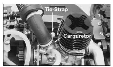
☐ 44. Place the air filter onto the carburetor. Using the remaining included tie-strap, tightly secure the air filter to the carburetor. Cut the excess portion of the tiestrap off to avoid interference.
