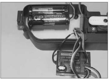
☐ 17. Install the receiver battery into the radio box. Note the placement of the receiver battery in the box. Connect the receiver battery to the remaining end of the on/off switch.
