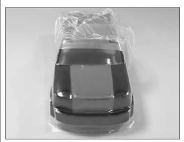
☐ 12. Remove the plastic from the outside of the body. Apply the decals to the body if desired.
