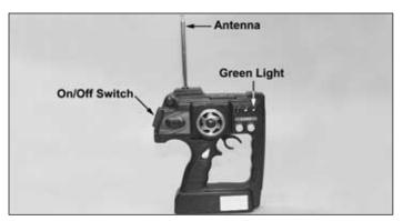
☐ 9. Remove the transmitter antenna from the holder and screw it into the hole on top of the transmitter.
