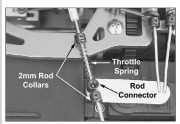
☐ 47. Tighten the rod collar that retains the throttle spring so that the spring cannot move back and forth but not so much that the spring is tight. The rod collar at the other end of the throttle linkage should be tightened against the rod connector as shown.
