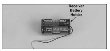
☐ 7. Remove the receiver battery holder from the radio box. Install (4) "AA" batteries (included) into the battery holder in the configuration molded into the battery holder.
