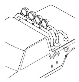
☐ 4. Drill six 1/4" (6mm) holes in the body using the molded-in dimples as guides. Install the rollbar onto body as shown using six 2.6 x 6mm self-tapping screws and the included collars.
