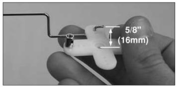
□ 3. Insert the brake rod as shown in the photo. Insert the brake rod into the servo arm from the bottom, into the second hole from the outside of the arm (approximately 5/8" or 16mm from the center).
