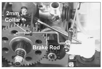
☐ 6. Install a 2mm collar at the end of the brake rod and another 2mm collar at the end of the throttle rod. Place a small amount of thread locking compound on two of the (3) 3 x 3mm set screws and thread them into the 2mm collars. Do not tighten the set screws all the way. In the next section we will make adjustments to the collars.
