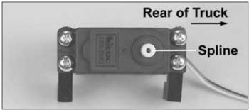
2. Attach the servo mounts to the steering servo with (4) 3 x 8mm self-tapping screws. Note that the servo spline will mount towards the rear of the truck.
