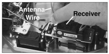
☐ 2. Remove the twist-tie from the receiver antenna. (The receiver antenna looks like a bundled thin wire that is attached to the receiver.) Thread the receiver antenna underneath and through the hole in the radio plate next to the receiver switch.
