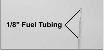
□ 3. Remove the antenna tube from the parts bag. Thread the receiver antenna through the antenna tube. The antenna will be longer than the antenna tube. **DO NOT COIL OR CUT THE ANTENNA.** Press fit the antenna tube through the hole in the radio plate. Place a 1/8" long piece of fuel tubing over the antenna tube and wire to secure in place. **TIP:** Run the antenna through your fingers to straighten out kinks before running through the antenna tube.
