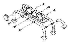
☐ 3. Assemble the rollbar as shown using ten 2.6 x 6mm self-tapping screws.
