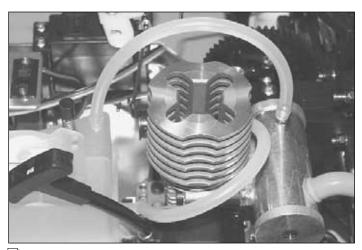
☐ 3. Cut the fuel line in half. Route one of the lines from the nipple on the top of the muffler to the top of the fuel tank. Route the other fuel line from the nipple on the carburetor to the bottom of the fuel tank. Ensure that the fuel line is not kinked anywhere along the line. You may have to shorten the line to eliminate kinks.
