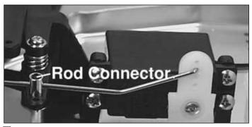
■ 8. Slip the steering rod through the hole in the rod connector that is already installed on the servo saver. (Use the screw that came with your radio system to attach the servo arm to the steering servo.) Do not tighten the set screw on the rod connector. You will make the steering adjustments later.
