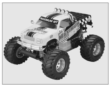
☐ 7. Mount the body on the body posts and secure the body to the truck with (4) body clips.
