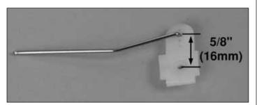
☐ 6. Put the steering rod into the third hole from the center of the servo arm (approximately 5/8" or 16mm). You may need to enlarge the hole in the servo arm with a 5/64" (2mm) drill or a hobby knife.
