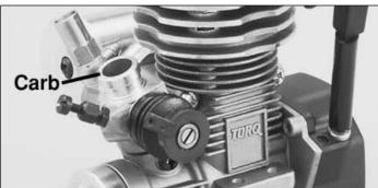
□ 4. Remove the air filter and tie strap from the parts bag. Thoroughly soak the air filter foam with some oil (not included) and then squeeze out the excess oil. A light machine oil (like 3-IN-ONE™) will work well. Special oils made for air filters are also available in most hobby and motorcycle shops. Place the air filter onto the carburetor and secure it in place with the tie strap. Cut off the excess part of the strap.
