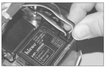
☐ 7. Plug the steering servo, throttle servo, and switch into the receiver. See your radio instructions to determine which channel is steering and which channel is throttle. The receiver switch plugs into the socket labeled "Battery," "Batt," or "B."
