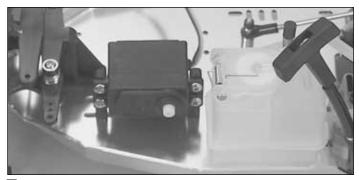
☐ 3. Attach the steering servo assembly to the chassis with (4) 3 x 8mm self-tapping screws in the holes provided as shown above.
