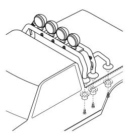
$\Box$  13. Drill six 1/4" (6mm) holes in the body using the molded-in dimples as guides. Install the rollbar onto body as shown using six 2.6 x 6mm self-tapping screws and the included collars.
