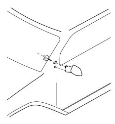
☐ 6. Drill one 1/8" (3mm) hole in each side of the body using the molded-in dimple as a guide, and one 5/64" (2mm) hole 7/16" (11mm) below and 7/16" back from first hole (use the pegs on the mirror as a guide). Install the mirrors as shown with the collars provided.
