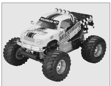
16. Remove the body clips from the parts bag. Place the body on the body mounts. On each body mount place a body clip.
