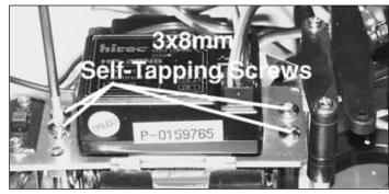
■ 8. Attach the radio tray to the radio tray posts with (4) 3 x 8mm self-tapping screws.
