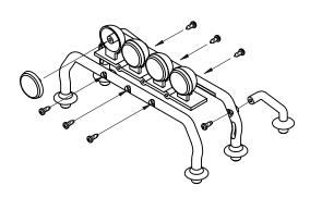
☐ 12. Assemble the rollbar as shown using ten 2.6 x 6mm self-tapping screws.
