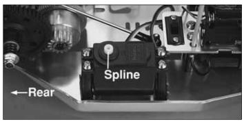
☐ 3. Use the (4) 3 x 8mm self-tapping screws to attach the throttle servo and the mounts to the chassis. Make sure that the servo spline is towards the rear.
