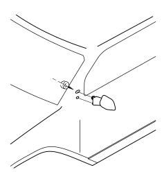
☐ 15. Drill one 1/8" (3mm) hole in each side of the body using the molded-in dimple as a guide, and one 5/64" (2mm) hole 7/16" (11mm) below and 7/16" back from first hole (use the pegs on the mirror as a guide). Install the mirrors as shown with the collars provided.
