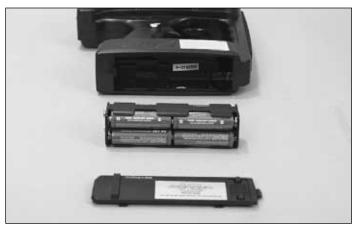
□ 9. Slide open the battery door on the bottom of the transmitter and remove the transmitter battery holder. Place 8 "AA" batteries into the holder in the configuration molded into the plastic on the battery holder. Re-install the transmitter battery holder into the transmitter and re-install the battery door.
