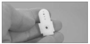
☐ 5. Use a 3 or 4 hole servo arm from your radio system. A 1, 2, or 4-armed servo arm will work. Cut off all but one of the arms by scoring both sides of the servo arm with a hobby knife and using pliers to snap off the arm.
