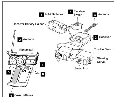
Before installing the radio system in the pre-built DuraTrax Maximum MT, read the manufacturer's instructions manual and follow the instructions shown below.
