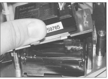
☐ 5. Remove the four screws from the top of the radio plate and remove the receiver battery holder.
