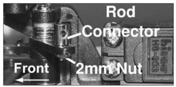
☐ 7. Place the rod connector through the top of the middle hole in the steering arm. Place a small amount of thread locking compound onto the threads of the rod connector. Do not to overtighten the nut, the rod connector must swivel freely. Install the 2mm nut onto the bottom of the rod
