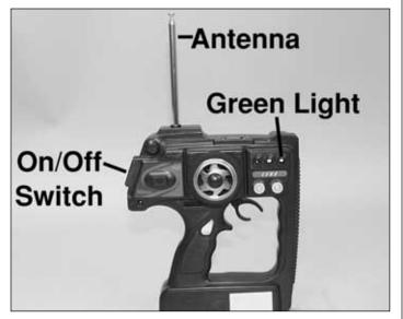
■ 8. Remove the transmitter antenna from the holder and screw it into the hole on top of the transmitter.
