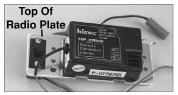
☐ 4. Attach the switch from your radio system so it is above the top of the radio plate (make sure the switch is in the OFF position). Remove the two screws on the top of the switch. Place the switch plate on top of the radio tray, the switch body on the bottom of the radio tray and then reinsert the screws from the top.
