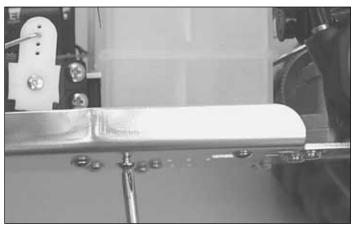
1. Remove the fuel tank by taking out the two screws on the bottom of the chassis.
