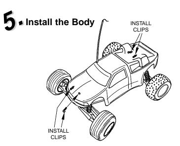
Place the body onto the chassis. Use clips to secure the body in place.
