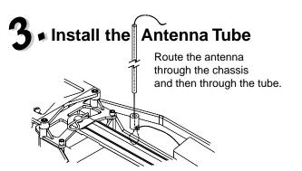
Install the antenna to the chassis. Secure excess wire to the tube using tape. **DO NOT CUT THE ANTENNA WIRE!!!**
