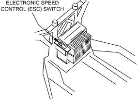
Turn on the switch in the chassis located next to the Electronic Speed Control (ESC).
