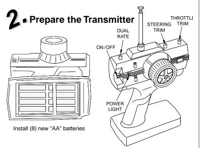
Screw in the transmitter antenna and install the "AA" batteries. Check to make sure the red power light glows when turning the switch "on".
