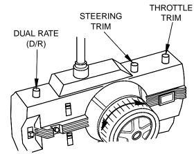
To make your Evader drive in a straight line, you may need to adjust the steering trim knob located on the transmitter. Adjust the dual rate knob to increase or decrease the steering travel. When first learning to drive, adjust the dual rate knob for less steering travel. As you get to be a better driver, adjust the dual rate knob for more steering travel.
