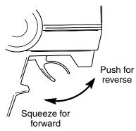
Hold up the rear wheels and squeeze the trigger. The rear wheels should spin forward. Push the trigger back. The rear wheels should spin backwards. If the wheels spin with the trigger in the neutral position, adjust the throttle trim knob located on the transmitter.
