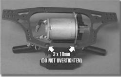
**5.** Install one of the chassis side plates onto the skid plate using two 3x18mm screws.
