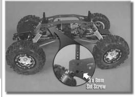
**19.** Install the body mount assemblies between the chassis plates and secure them in place with the shock mounts and one 3x8mm set screw on each side.
