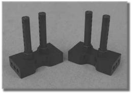
**18.** Trim the locating tab from the bottom of the stock MRC body mount posts. Install the body posts onto the Mini GC3 body mount braces using the included 2x14mm flat head screws.
