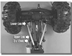
**17.** Install the front axle assembly to the chassis. Attach the upper links to the outside of the chassis plate and secure them in place using two 3x12mm screws and two 3mm lock nuts. Attach the lower links to the front axle.
