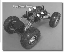
**20.** Install the upper chassis braces and secure them with 3x8mm screws.
