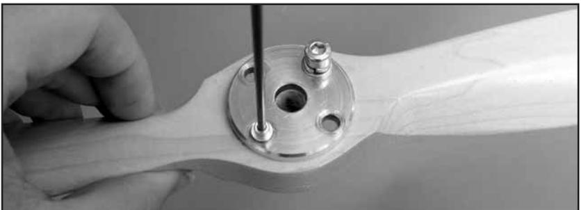
7. Use one of the 5x40mm SHCS with 5mm lock washers and 5mm flat washers to align the propeller washer on the propeller and use the Dead Center Hole Locator to mark position of the remaining holes.
