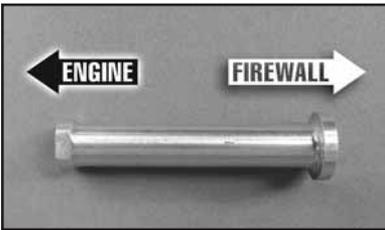
2. Install the standoffs to the engine with the included (4) 5 x 25mm SHCS and 5mm flat washers (it's a good idea to use 5mm lock washers between the SHCS and the flat washers). Next, install the engine with standoffs to the firewall using (4) 5 x 20mm
