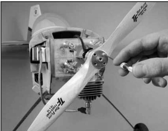
**5.** Mark the location of one of the outer holes while the propeller is in the beginning of the compression stroke position. Use a GPM Dead Center Hole Locator (GPMR8130) to center and start the hole.
