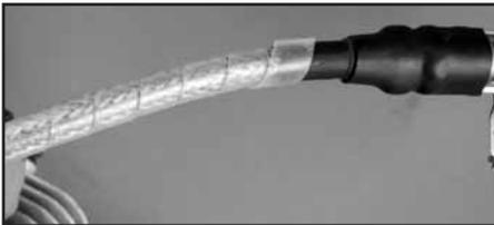
**5.** Install the silicone ignition wire covers over the ignition wires.
