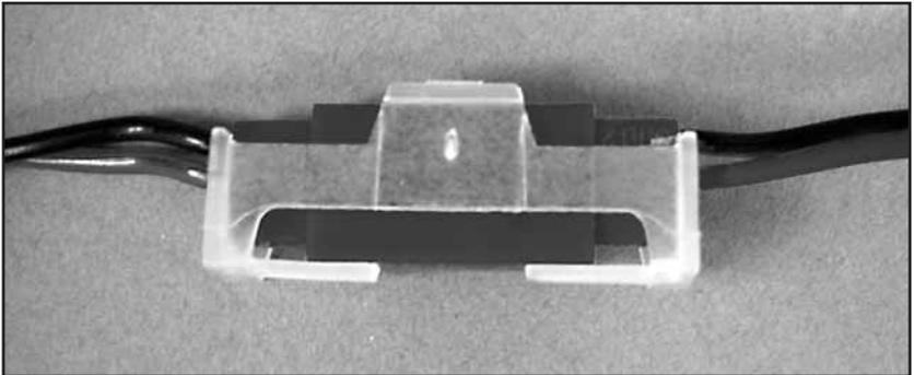
**3.** Connect the ignition kill switch lead to the red connector from the ignition control module using the lead from the kill switch or with the included three pin connector with pig tail. Use the included three pin securing clip to secure the connection.
