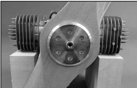
4. Place the propeller on the crankshaft at the one o'clock position.
