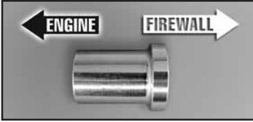
2. Install (4) 6mm blind nuts or tee nuts (not included) into the back side (non-engine side) of the firewall. Install the engine to the firewall using (4) 6x45mm SHCS with 6mm lock washers and flat washers (not included) with the included standoffs. Use some threadlocking compound, such as Great Planes® Pro™ Threadlocker (GPMR6060) on the screws where the threads enter the blind nuts.
