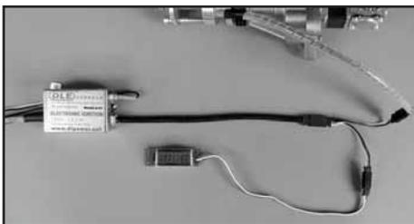
Many of the DLE Ignition modules have an additional lead to plug into the optional tachometer. If your ignition module does not have this additional lead, the digital tachometer can still be used. Simply use the Y-harness
