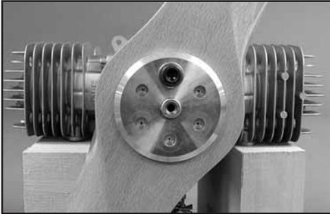
6. Remove the propeller from the engine and drill the outer hole on the drill press using a #35 (.110"/2.81mm) drill bit as a pilot hole. Next use a 1/4" (6.28mm) drill bit to finish the hole. In order to achieve a clean finish on both sides of the propeller drill only half way through
