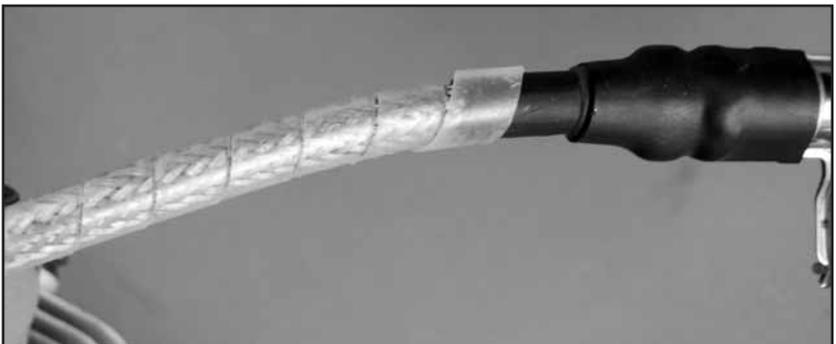
**5.** Install the silicone ignition wire cover over the ignition wires to the spark plugs.
