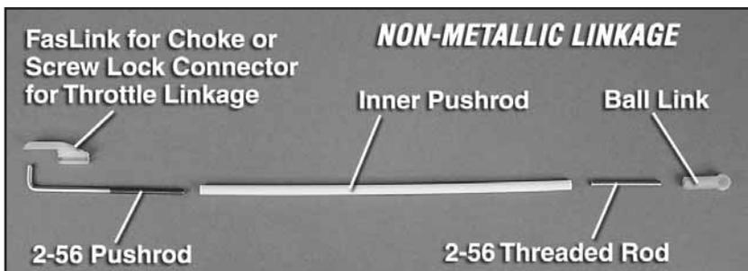
5. Install the throttle servo and choke servos at least 12" [305mm] away from the engine. Make sure that you get the throttle and choke's full range of rotation with your servos travel. Be sure to use a non-metallic linkage for both the throttle and choke linkage. A high-torque heavy duty metal gear servo is recommended to operate the throttle on the DLE-170. (Components for the non-metallic linkage can be purchased through your local hobby shop.)
