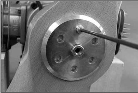
5. Mark the location of one of the outer holes on the propeller. Use a GPM Dead Center Hole Locator (GPMR8130) to center and start the hole.
