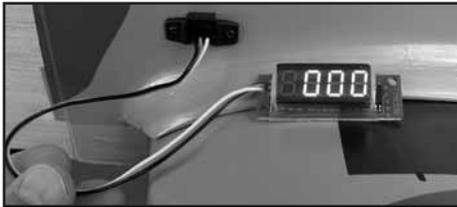
An optional digital tachometer is available that can be directly connected to the ignition and display the RPMs of the engine. This unit can be installed on the aircraft or used to spot check
