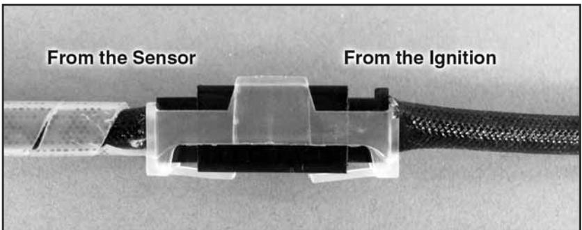
2. Install the silicone wire cover over the pick up lead coming from the engine (cut the excess silicon wire covers) and connect the lead to the pick-up lead from the Electronic Ignition Module. Secure the connection with the included three pin connector securing clip.
