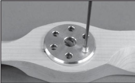
**6.** Remove the propeller from the engine and drill the outer hole using a #35 drill bit as a pilot hole. Next use a #5 (.2055" / 5.21mm) drill bit to finish the hole. In order to achieve a clean opening on both sides of the propeller, drill only half way through
