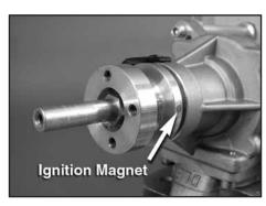
3. Next, set the engine at the beginning of the compression stroke. Note the position of the ignition magnet with engine inverted.
