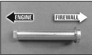
2. Install the standoffs to the engine with the included 5 x 25mm SHCS and 5mm flat washers (it's a good idea to use 5mm lock washers between the SHCS and the flat washers). Next, install the engine with standoffs to the firewall using (4) 5 x 20mm SHCS with 5mm
