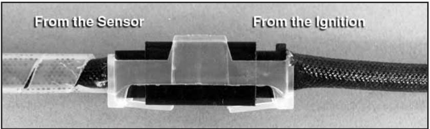
2. Install the silicone wire cover over the pick up lead coming from the engine (cut the excess silicon wire cover) and connect the lead to the pick-up lead from the Electronic Ignition Module. Secure the connection with the included three pin connector securing clip.
