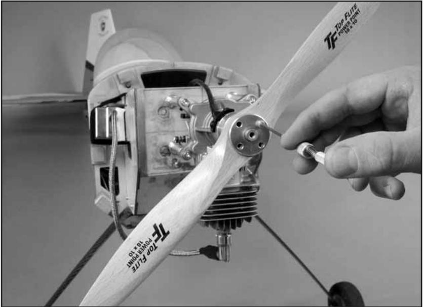
5. Mark the location of one of the outer holes while the propeller is in the beginning of the compression stroke position. Use a GPM Dead Center Hole Locator (GPMR8130) to center and start the hole.
