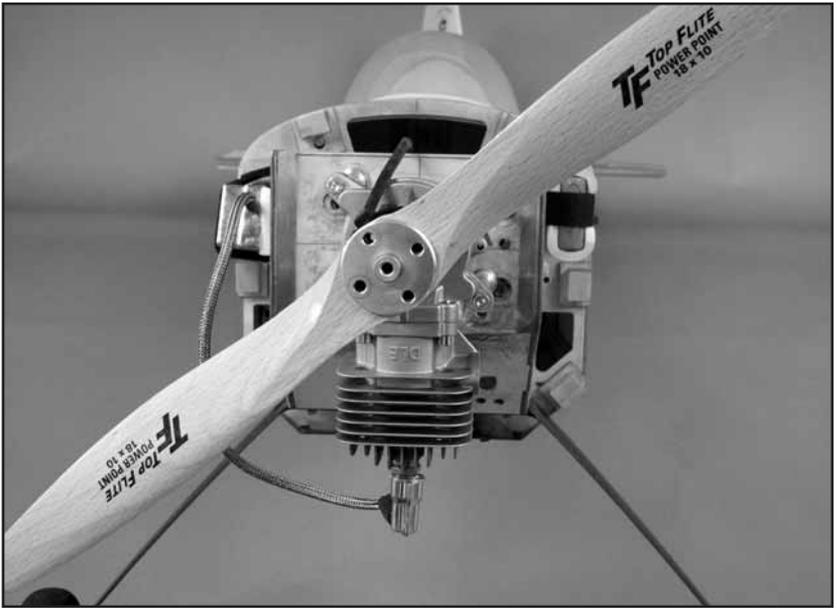
4. Place the propeller on the crankshaft at the one o'clock position.
