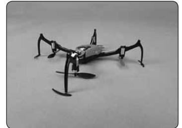
Unlike your typical multi-rotor craft, the Verso is capable of taking off upside-down or flipping itself inverted during flight with the press of a button and then continuing to fly normally. Sensors on the Verso automatically detect which side of the quad is facing up and will adjust the rotation of the motors accordingly. Because of this feature, there is some functionality that is unique to the Verso:
