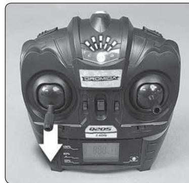
1. Turn on the controller with the left stick at its lowest position. The LED on the controller will flash, indicating it is waiting for the arming sequence.
