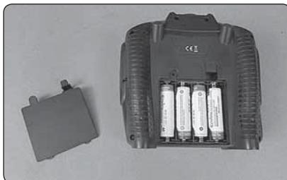
Remove the battery cover to insert the included (4) AA batteries. Reinstall the battery cover.
