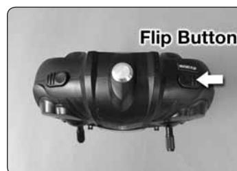
The default setting for the flip function is 180°. To change the flip function to 360°, press and hold the flip button for at least two seconds. The transmitter beeps once for 180° mode and beeps twice for 360° mode.
