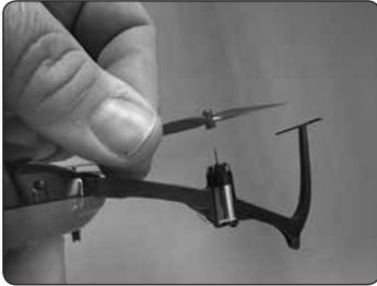
If a rotor blade needs replacement, use the prop removal tool or a thin, flat bladed screwdriver to pry off the damaged rotor blade. The new blade can be pressed onto the motor shaft with just finger pressure. Take care not to bend the replacement rotor blade when installing.
