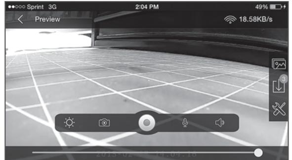
1. To activate the “record” function, simply push and release the **Video On/Picture Button** on the back/right hand side of the controller.
