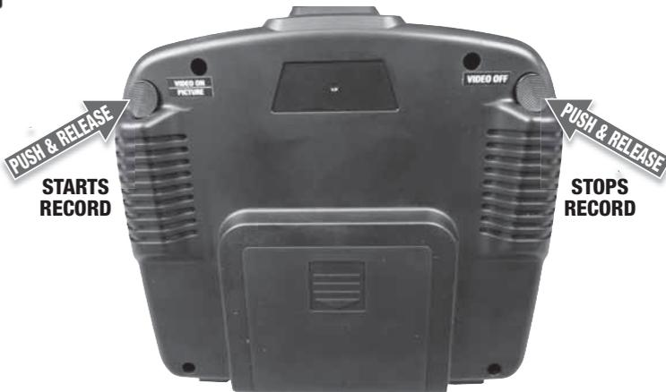
1. To activate the “record” function, simply push and release the **Video On/Picture Button** on the back/right hand side of the controller.
