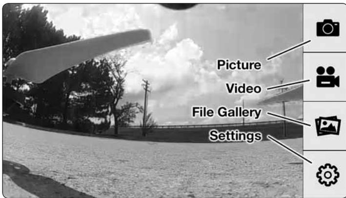
6. Once connected you will see on your device the image seen by the camera (referred to in this manual as the FPV feed). Press anywhere on the screen to pull up the main options.
