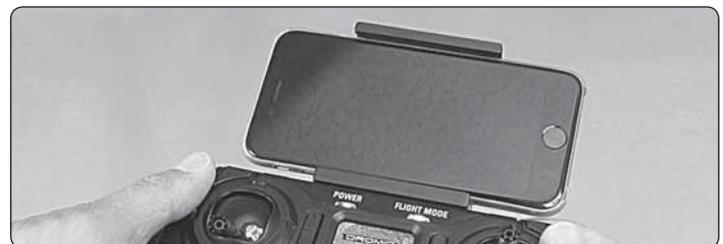
4. Grasp your device as shown and attach it to the phone mount on the controller by pushing up on your phone against the spring loaded top clip until you can fit the other side into the bottom clip.
