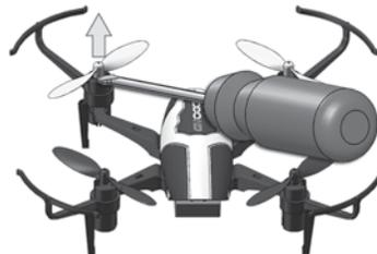
1. Carefully pry off the blade using a flat head screwdriver. **NOTE:** Do one corner at a time so you don't accidentally mix up the blades.
