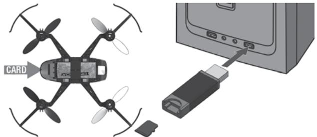
Only insert and remove the memory card when the battery is not connected to the Kodo HD. When the memory card is installed, there will be a steady blue LED just above the card slot.
