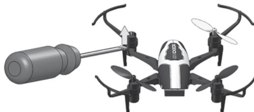
2. Pull blade guard up and off the motor housing. Install the new guard and replace the rotor blade.
