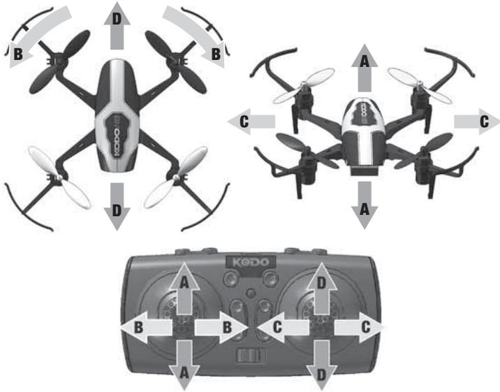
**Basic Flight** Advance the throttle slowly until your Kodo HD rises into the air. The controls are very sensitive and small stick movements should be used to control the quadcopter. If you get into trouble and see that the Kodo HD is going to crash, move the throttle to its lowest position immediately.
