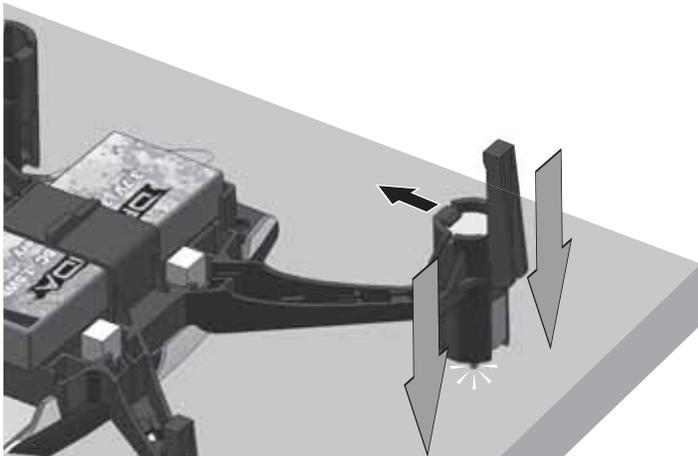
1. Remove the rotor blade from the motor.
