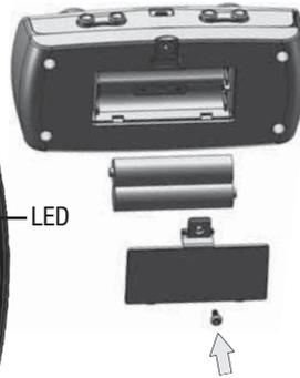
Remove the screw on the battery compartment cover. Take the cover off and insert 2 AAA batteries. Replace cover securing with the screw.
