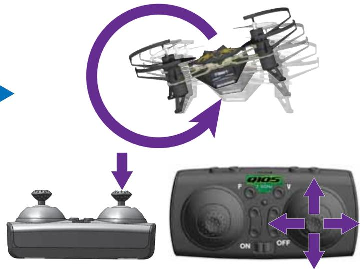
Push down on the right stick and release it to start the flip. Hold the right stick in any direction and release it when the flips are completed. The radio will beep until the right stick released.
