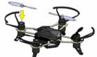
3. Push the prop onto the motor so it is tight on the shaft.
