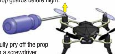
1. Carefully pry off the prop using a screwdriver.
