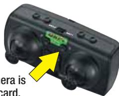
To capture a photo, press the "P" button. The red LED on the quad will flash once to indicate that a photo has been captured and stored. The camera will not capture a photo while it is recording a video.
