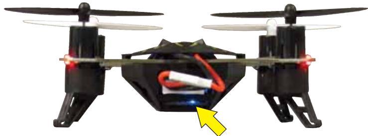
Please disconnect the battery before the memory card is inserted or removed from the camera. When KODO is linked with the controller and the card is installed correctly, there will be a steady blue LED just above the card. A red LED flashing next to the blue LED when the camera is not operating indicates that the card is missing or not installed correctly.
