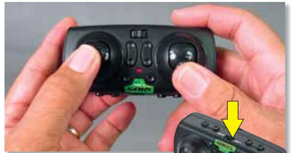
For Mode 1 operation, slide the mode switch to the MD1 position and hold the controller with the throttle on the right side.
