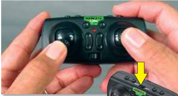
For Mode 2 operation, slide the mode switch to the MD2 position and hold the controller with the throttle on the left side.
