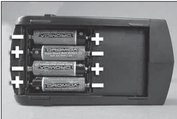
Insert 4 "AA" batteries into the bottom of the radio.
