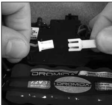
1. Install the battery into the vehicle and connect the battery.
