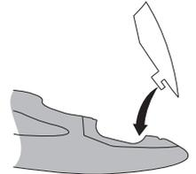
5. Rotate the back of the canopy onto the latch and apply pressure. There will be a 'click' when the latch is secure.
