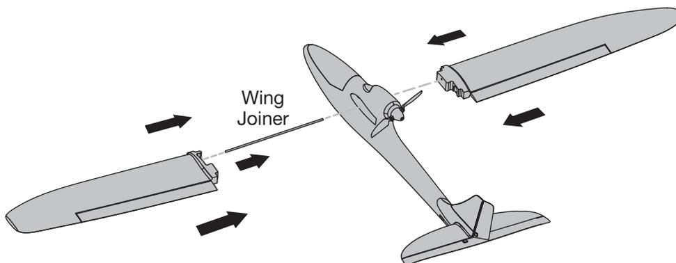
Insert the wing joiner into one of the wing halves. Next, slide the two wing halves together inside the fuselage as shown.
