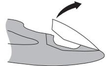
3. Connect the matching plugs and install the battery in the nose of the plane.
