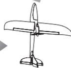
2 Once the turn starts, add in a small amount of up elevator to maintain altitude and help turn the plane.
