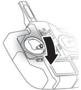
2. Undo the canopy latch. Lift up on the back edge of the canopy and then slide it backwards.
