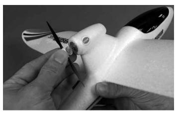
Press the propeller onto the propeller base attached to the motor shaft. Press firmly until it clicks into place. If the propeller does not easily snap into place, rotate the propeller slightly to align the splines on the base.
