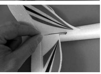
2. If additional trim is required beyond what the trim buttons are capable of making, the clevises can be disconnected from the control horns and threaded forward or aft on the pushrods. This will allow the control surfaces to be centered with the trim buttons at or near the center position.
