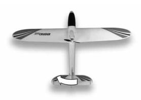
When the left control stick is in the down position, the propeller will not rotate. To test the operation of the motor, be sure to have a firm grasp of the airplane with your hands clear of the rotational arc of the propeller. Be sure to point the propeller away from people or obstructions.
