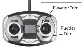
1. Before making your first flight, use the trim buttons to center the elevator and rudder surfaces. Adjust the trim as necessary using the trim buttons until the control surfaces are inline as shown.
