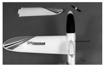
Insert the wing into the fuselage.
