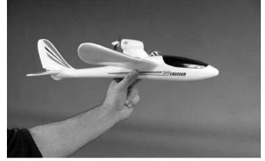
making the first turn (away from yourself). Do not "yank" back the elevator stick forcing the plane into too steep of a climb. This could cause the model to quit flying and stall.
