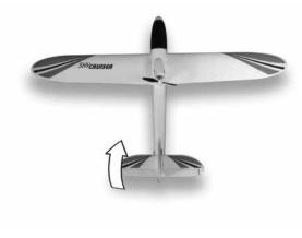
When the right control stick is moved to the left, the rudder will move to the left.
