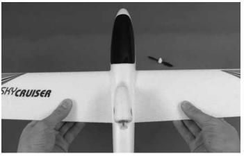
Fit the other wing panel onto the carbon rod. Push the wing panels together.
