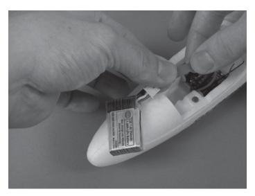
Connect the battery to the plane and insert the battery into the slot at the front of the fuselage. Be sure the battery wires do not contact the servo gears in the fuselage. The motor is now considered live. Keep clear of the propeller in case of accidental start-up.
