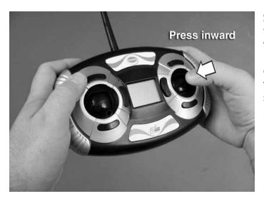
Select the desired skill mode by pressing inward onto the elevator/rudder control stick. If this is your first time flying the Sky Cruiser, select the Low Rate mode. This will provide reduced control throws to lessen the chance of over-control for your first flights. As you become proficient flying the Sky Cruiser, experiment with the high rate setting at a safe altitude.
