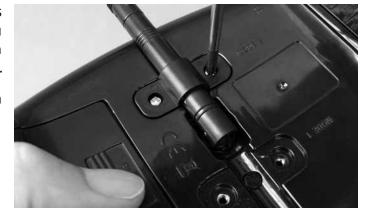
Rotate the antenna upward until it is vertical.
