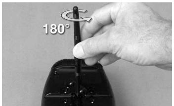
Fold the antenna back down into the other side. Reinstall and tighten the (2) mounting screws.
