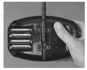
Turn on the power switch on the transmitter and observe the battery icon in the status display. When the battery icon is blinking, the batteries are too low and should be replaced. Four squares inside the battery icon indicate that the batteries are at full power.
