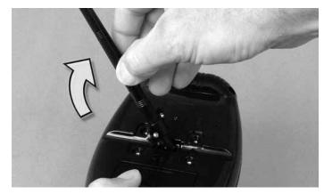
Rotate the antenna 180°, allowing it to be folded down the other way.
