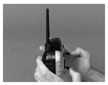
Be certain the transmitter antenna is in its vertical position and that the power switch on the transmitter has been turned on. **Note:** Unless performing the "Binding" procedure described on page 9, never allow the battery to be connected to the Sky Cruiser without the transmitter turned on. This means you should always turn on the transmitter first before installing the battery into the model, and always turn off the transmitter first before removing the battery from the Sky Cruiser.
