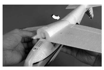
Insert the plastic tab at the aft end of the wing into the fuselage as shown, ensuring that the wires are inside the fuselage and do not interfere with the other servos.
