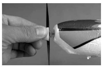
Press the propeller onto the propeller base attached to the motor shaft. Press firmly until it clicks into place. If the propeller does not snap easily onto the propeller base, rotate the propeller slightly and try again.
