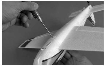
Press the wing into position and use the screw you removed from the wing hold down bracket to secure the wing in place. Do not over tighten the screw.
