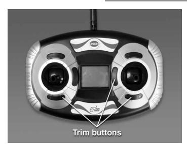
With the power switch on the transmitter turned on, press the trim buttons as necessary to center the trim indicators in the status display.
