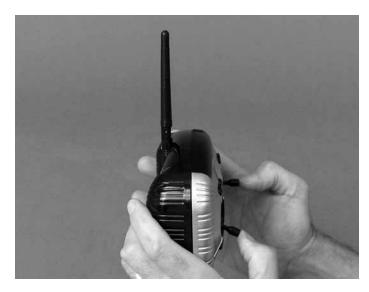
Be certain the transmitter antenna is in its vertical position and that the power switch on the transmitter has been turned on. **Note:** Unless performing the "Binding" procedure described on page 9, never allow the battery to be connected to the Extra without the transmitter turned on. This means you should always turn on the transmitter first before installing the battery into the model, and always turn off the transmitter first before removing the battery from the Extra 300.
