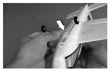
Insert the landing gear into the slot behind the battery compartment. Be sure the gear is pressed into the slot completely.
