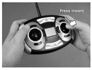
Select the desired skill mode by pressing inward onto the elevator/aileron control stick. If this is your first time flying the Extra 300, select the Low Rate mode. This will provide reduced control throws to lessen the chance of over-control for your first flights. As you become proficient flying the Extra, experiment with the high rate setting at a safe altitude.
