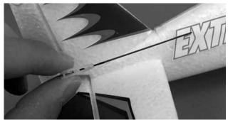
The ailerons can be adjusted in the same manner by disconnecting the ball links. When setting up the trims for the first flight, be sure that you will have trim movement available in both directions so you can make fine adjustments during the flight.
