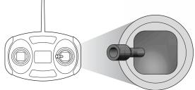
When the left control stick is moved to the left, the rudder will move to the left.
