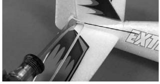
2. If additional trim is required beyond what the trim buttons are capable of, the clevises can be disconnected from the control horns and threaded forward or aft on the pushrods. This will allow the control surfaces to be centered with the trim buttons at or near the center position.
