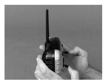
Be certain the transmitter antenna is in its vertical position and that the power switch on the transmitter has been turned on. **Note:** Unless performing the "Binding" procedure described on page 9, never allow the battery to be connected to the Sky Ranger without the transmitter turned on. This means you should always turn on the transmitter first before installing the battery into the model, and always turn off the transmitter first before removing the battery from the Sky Ranger.
