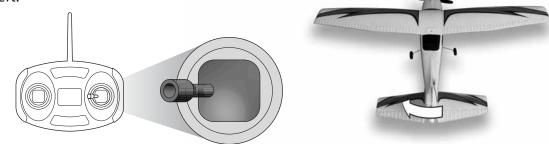
When the left control stick is in the down position, the propeller will not rotate. To test the operation of the motor, be sure to have a firm grasp of the airplane with your hands clear of the rotational arc of the propeller. Be sure to point the propeller away from people or obstructions.
