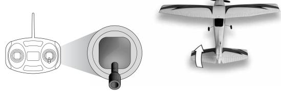
When the right control stick is moved to the left, the rudder will move to the left.
