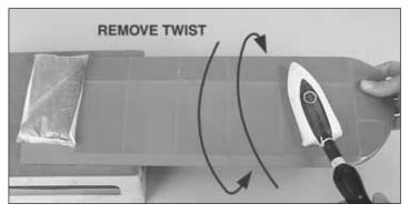
12. After the model has been covered, check the wing and tail for any undesirable twist. Twist can be removed (or added if desired) by using weight to hold one end down and twisting the other end in the opposite direction. Heat the covering on the top and bottom until the wrinkles have disappeared. Check the result. Repeat if necessary.
