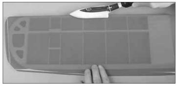
4. With your iron set to 175° - 195°F [70° - 80°C] start by bonding one edge of the covering to the framework-to the leading edge of the wing in this example.
