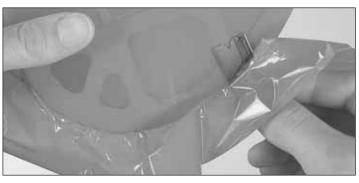
☐ 10. Use a sharp blade to cut the excess covering from the wing. Retrace your steps and iron down the seams all the way around.
