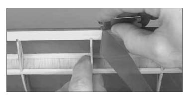
☐ 8. Use a sharp #11 blade or a single-edge razor blade to trim the excess covering from all the way around the framework. Re seal all the edges you cut to make sure it is thoroughly bonded to the framework.
