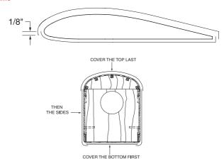
One way to a good covering job is to conceal seams where two pieces of covering overlap. Cover the bottom first, then wrap the top (or side if covering the fuselage) down around the bottom. When covering the fuselage, start with the bottom, then the sides followed by the top. Seams should overlap approximately 1/8" [3mm].
