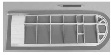
1. Start by covering the underside of the wing. Partially unroll the covering and lay the wing over it. Since the adhesive is on the back, and we are starting with the bottom of the wing, the covering should be upside-down, adhesive side up. Cut a piece of covering approximately 1" [25mm] larger than the wing all the way around.
