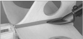
When covering horizontal and vertical stabilizers that have already been joined to the fuselage, fold a small strip of covering in half by making a crease down the middle. Use a trim iron to bond the strip to the stab and fin.
