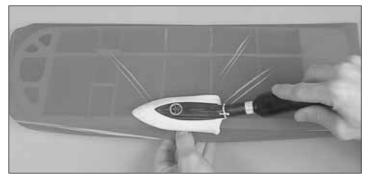
☐ 5. Lightly tug on the covering to pull out most of the wrinkles, then bond that area to the opposite side—in this example to the trailing edge. Perform the same procedure moving up and down the trailing edge until it is bonded to the wing.
