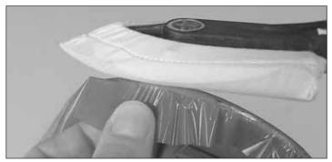
☐ 7. Use the iron to drag the covering up over the leading and trailing edges. When you get to curved areas like the wing tip, stretch the covering by pulling on it, then seal it to the framework. Don't let go until the covering has cooled for a few seconds and the adhesive has taken hold. Do little sections at a time.
