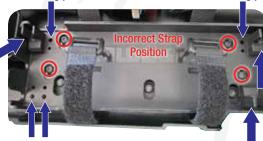
Using a 5/64" (2.0mm) hex driver remove the four 3x8mm button head screws that attach the battery tray to the chassis of the vehicle.
