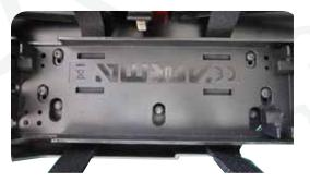
Insert the screws and loosely tighten them so that they do not fall out. Do NOT tighten.
