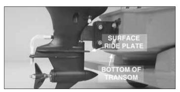
A template has been provided for you on page 3 of this manual. This will help to accurately place the mounting holes. Mount the outboard unit in the center of the rear of the boat and so that the surface ride plate is even with the bottom of the transom as shown.
