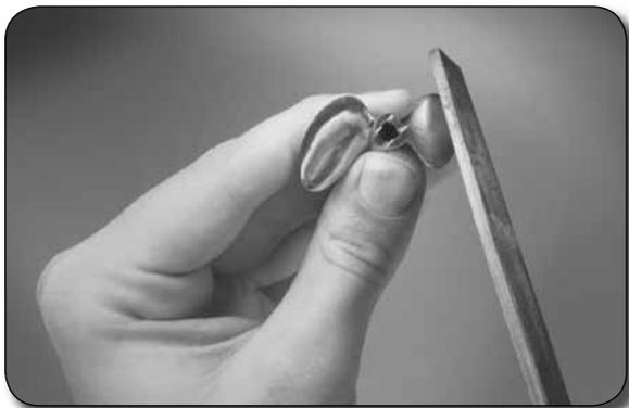
Use a flat file and work your way from the trailing edge to the tongue. Care has to be taken not to roll the leading edge of the propeller as you sharpen. Work slowly and take your time.
