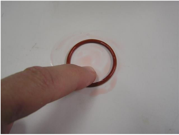
4. Coat O-ring with oil
