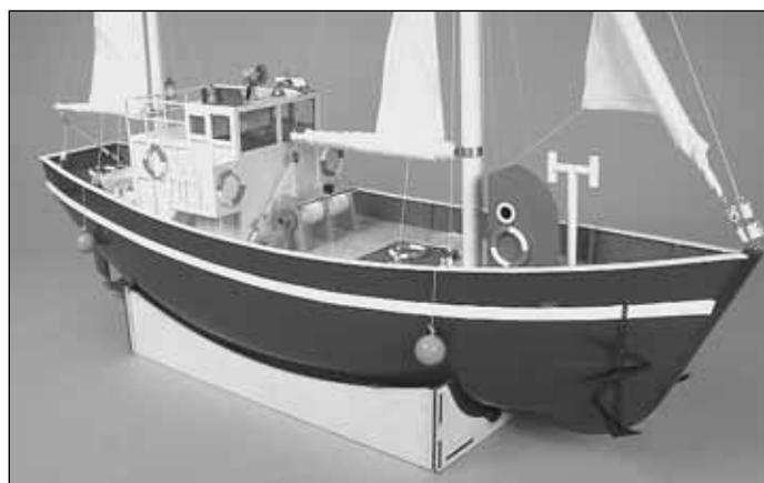
❑ 1. Turn the power “ON” to the transmitter and receiver (in that order). Attach the port (left) and starboard (right) cabin hooks to their retaining rings and carefully set the cabin in place as shown.
