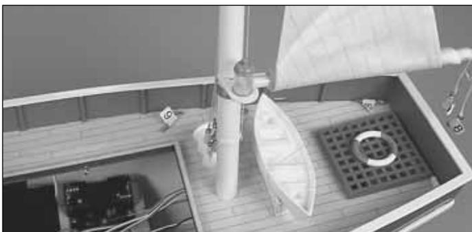
□ 4. Insert the rear mast into the round opening at the rear of the radio compartment opening. Gently twist the mast so that the running light is toward the port (left) side as shown. **Note:** Be sure that the receiver antenna is inserted into the rear mast before inserting the mast into the opening.
