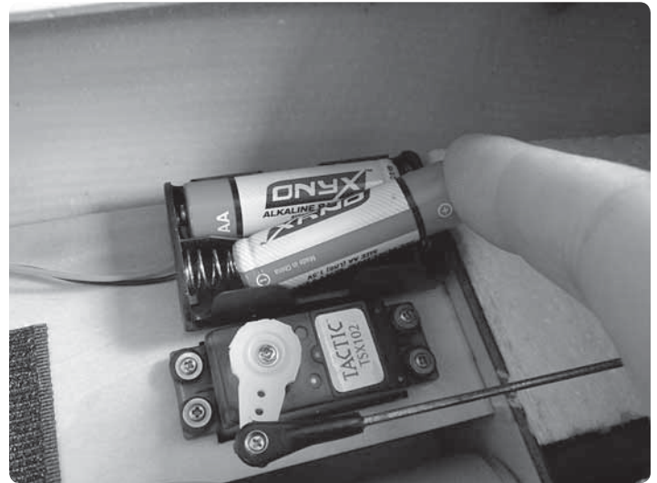
Next install two AA batteries into the battery holder located on the radio tray.
