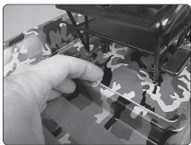
Rotate the lock and lift the front edge of the seat compartment. Slip the radio box cover forward and up. Then, place it to the side.
