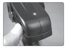
Turn the transmitter on, making sure the power light is glowing.
