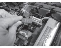
To turn the lights on and off, use the switch located on the side of the radio box.
