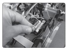
Install two AA batteries into the battery holder for the LED lights.
