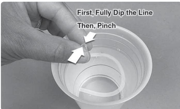
2. Fully submerge the line in water. Pinch the end closed as you remove the line from the water.
