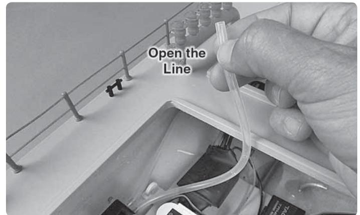
1. Remove the water line between the water pick up tube and water pump.
