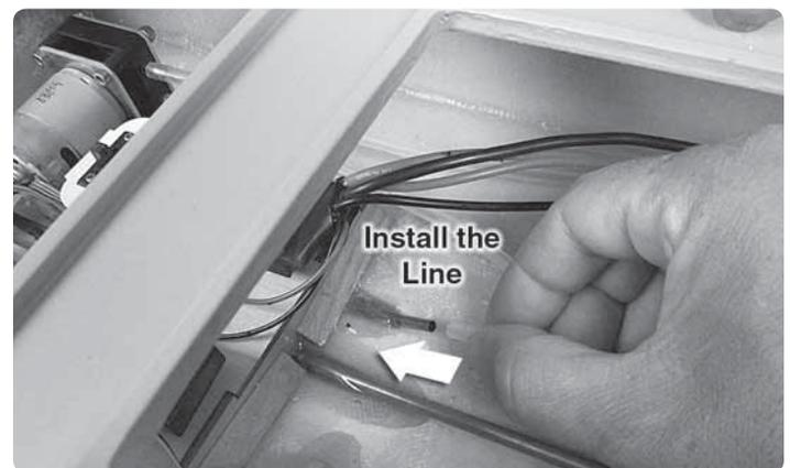
4. Install the open end of the line back onto the pickup.
