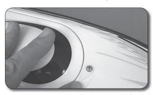
1. Remove the cowl by rotating the lock near the front of the windshield.
