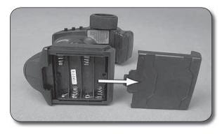
1. Slide off the battery door from the bottom of the transmitter.
