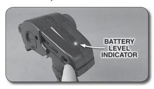
4. Turn the transmitter "ON" using the switch on the transmitter's left side. The battery level indicator light (LED) should glow red. If the light is flashing, the batteries are low and need to be replaced.
