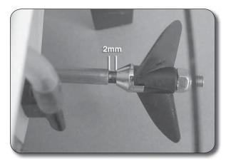
5. Leave about 1/16" [2mm] gap between the front of the drive dog and the back of the shaft tube.
