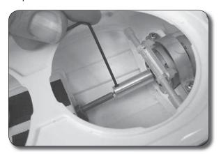
2. Using a 1.5mm Allen wrench, loosen the set screws holding the drive cable to the motor coupler. It is important to note that there are two set screws holding the cable in position.
