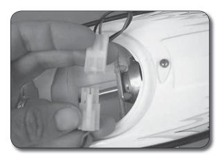
6. Install the hook and loop to the battery and install the battery in the boat. You will notice the plug can only be attached one way. Pay attention to the polarity of the plug. Plug the battery into the RX/ESC combo unit.
