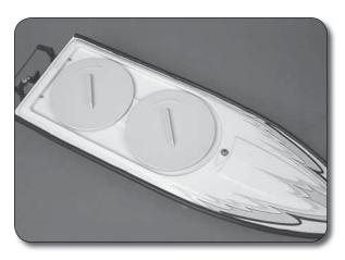
8. Re-install the covers by aligning the tabs on the bottom of the covers with the tabs in the openings. Rotate the covers 45° to secure them in place.
