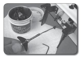
4. Using GrimRacer speed grease, apply a small amount to the cable and slide the cable back into the boat. Be careful to align the cable to the hole in the end of the motor coupler.
