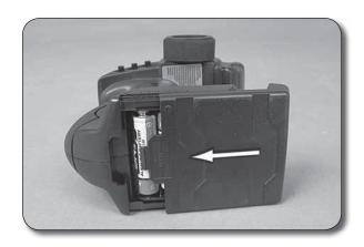
3. Reinstall the battery door onto the bottom of the transmitter.
