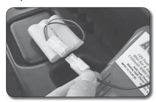
5. Join the battery and charger connectors. The connectors are designed to only connect one way to prevent the battery from being hooked up backwards.
