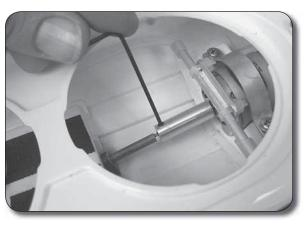
6. Tighten the set screws to hold the cable in place. Do not over tighten the set screws. It is also a good idea to tighten one screw lightly and then the other. Go back and forth between screws to keep even tension on the drive cable.
