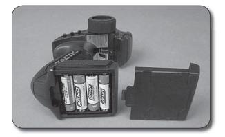
2. Install 4 "AA" batteries into the transmitter in the configuration molded into the battery floor.
