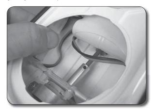
7. Tuck the battery plug under the deck of the boat to keep the wires away from the drive components. Make sure the battery pack and wire are NOT touching the drive components.
