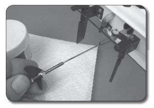
3. Slip the cable out the back of the boat. Wipe off any grease and water that might be on the cable.
